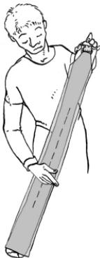
2. Place the ski on a stable surface, preferably a solid ski waxing table. Starting from the tip, use the POMOCA cutter to carefully trim the skin along the edge opposite to you. The cutter cuts the skin leaving automatically 2mm free edge.
